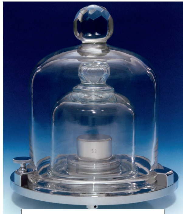
The "national kilogram" is the measure of mass and is available at the federal physical-technical institute PTB (picture: PTB).
